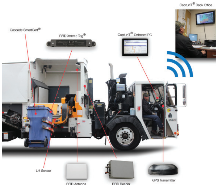
The RFID equipment used in an automated residential collection system. Images courtesy of Cascade Engineering.
